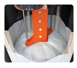
The inner bag is stretched and twisted at the same time. If needed, the procedure can be paused and resumed at a later stage.
