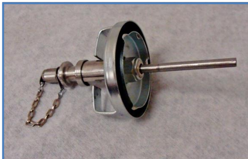
GE 788-SD-SC, Dipstick, sample point cap wheel motor
